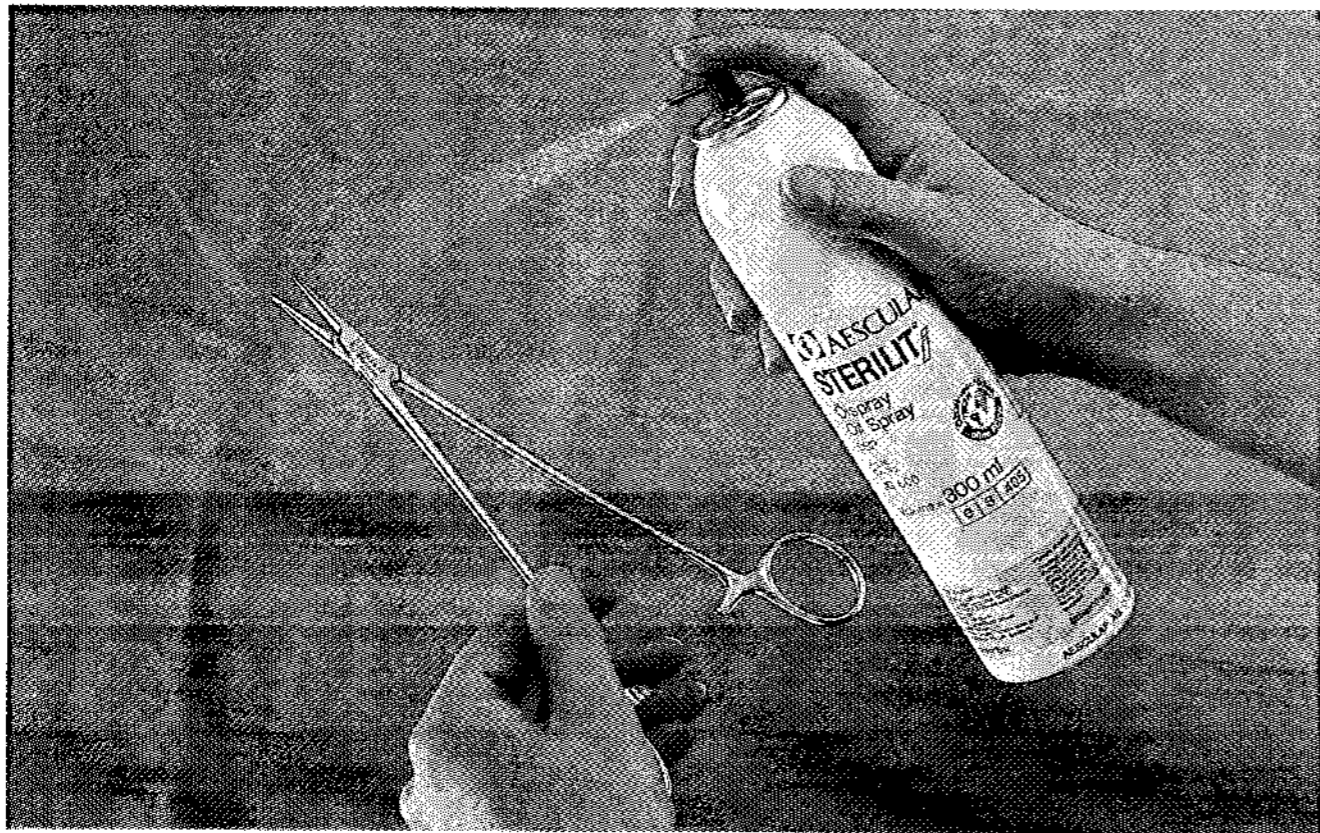
4.7. After thorough cleaning by a washing line or a washing machine, the instruments are oiled in the joint with a special oil to reduce friction and arranged in the tray in accordance with the packing list.
