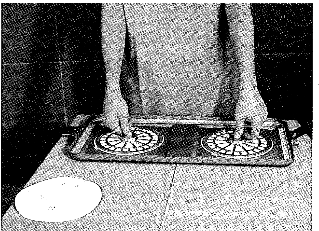
4.6. ... and the filter holders are brought to their original position by means of a pushbutton mechanism.
